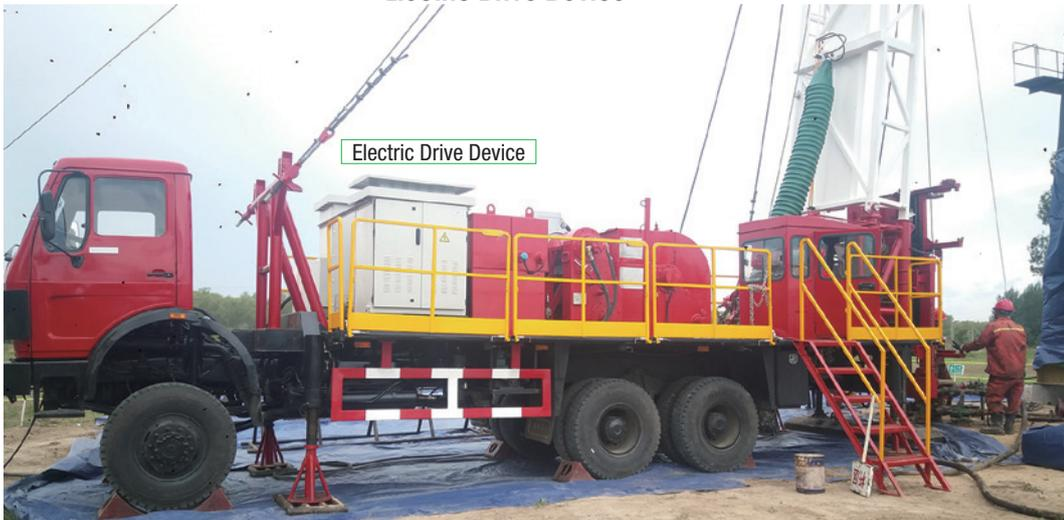
**Our fracking team used grid power for fracking in the Chuanqing downhole hydro-fracturing project.**
