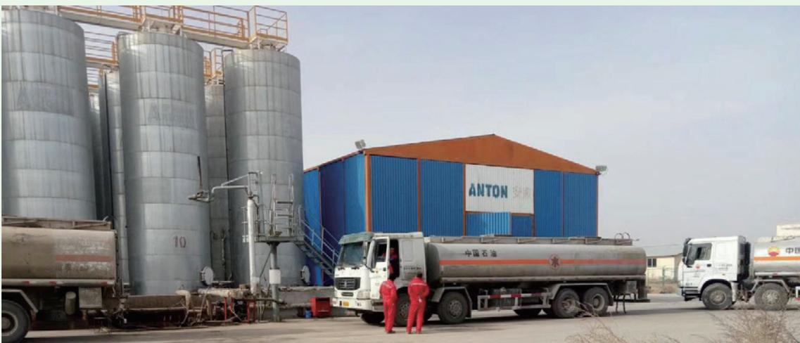
We established central mud stations (Suining in Sichuan and Tarim in Xinjiang) for areas with higher concentrations of engineering teams to enable the recycling of oil-based mud.
